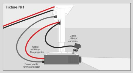
3) USB cable to connect the camera to a PC, preferably use active, with good power transmission, or an ordinary cable, no more than 5 meters long.
