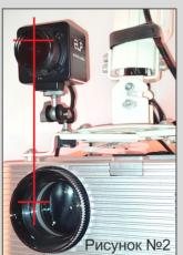
Mount the camera firmly above the lamp projector using a convenient latch, as shown in picture Nº2.
